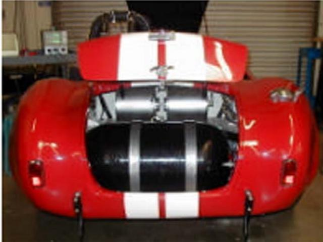
Figure 7 – Hydrogen storage tank
