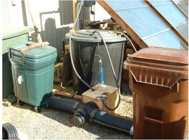
11. The indicated temperature of the wood chip container on this 65-degree day averaged 104 degrees. Solar heated water to the radiator was 156 degrees producing 108 degree hot air at the entry point to the dryer. Moisture content of the wood is reduced to 10-15% most days of the year.
