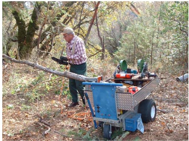
6. Here Ed has dropped in the fireplace size 16” sections into an electric powered bundler and is binding them together with a very tough adhesive backed strapping tape. Note the handy fire extinguisher.
