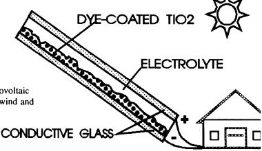
useful electrical current, and then the external circuit returns the electron to the other side of the cell, where it travels through the electrolyte back to the dye molecule.
