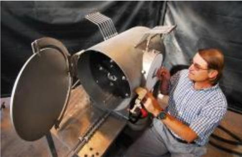
This mouth-full from Sandia National Lab uses a parabolic mirror to heat a chamber of water and nasty CO<sub>2</sub> to 1500° C, producing hydrogen, oxygen and carbon monoxide, precursors to synthetic fuel. They say it could be ready for market in 15 to 20 years. If people keep up this sort of thing, we may never see that \$20 a gallon gasoline.
