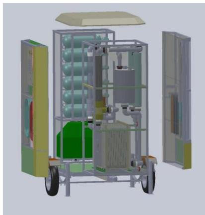
After several years of development and gallons of blood, sweat and tears, the Hysolgenics solar EL-5000 electrolyzer is finally producing hydrogen. The AHA has ordered one and it is now being mounted on a trailer for transport to Phoenix. It will produce about 1 cubic foot of H<sub>2</sub> per minute. See it at work:
