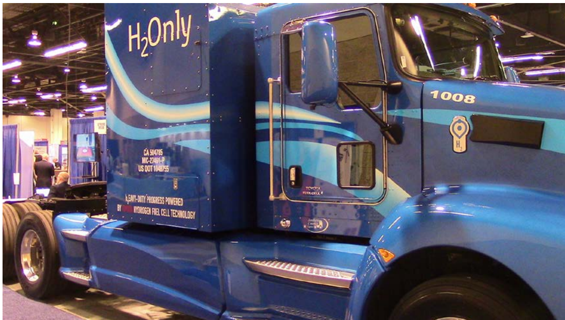
Toyota semi-truck powered by two Mirai fuel cells
